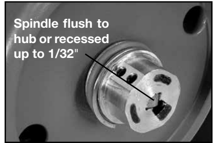
Figure 18 - Spindle Flush or Recessed
